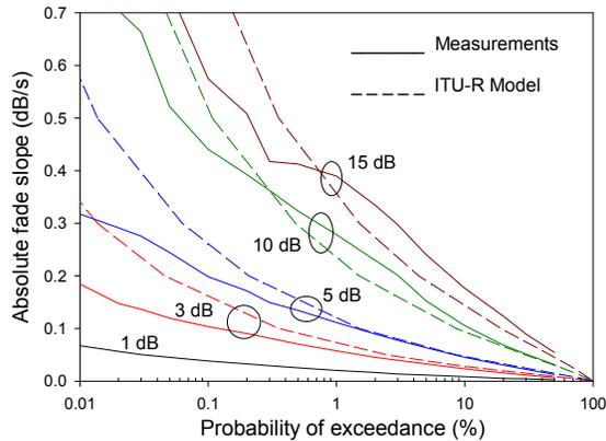
Fig. 5 Comparison of absolute fade slope CDFs derived from Anik F2 with the model in ITU-R Rec. P.1623 [4].
