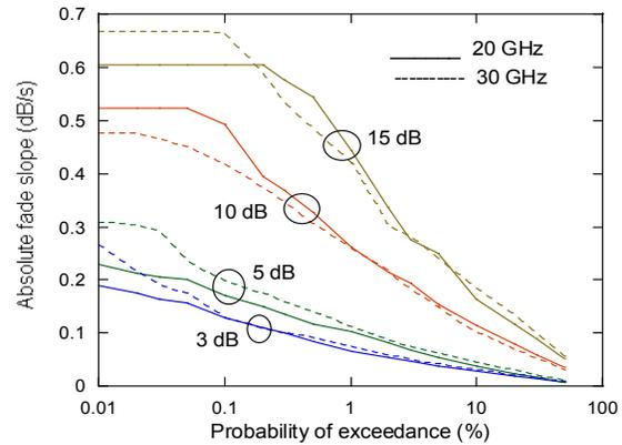
Fig. 6 Conditional CDFs of absolute fade slope from the 20 and 30-GHz ACTS satellite data collected at CRC during 4 years.
