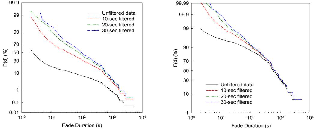
Fig. 1 Conditional CDFs of relative number of fades,  $P(d)$ , and of total fraction of fade time,  $F(d)$ , for an 8-dB fade threshold. Dashed lines show CDFs from data filtered using a raised cosine filter with 10-, 20-, and 30-s integration time.
