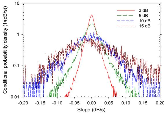
Fig. 3 Conditional PDF of fade slope for various different attenuation levels.
