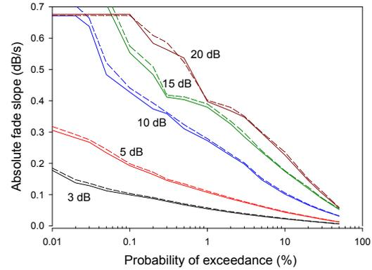
Fig. 4 Conditional CDF of absolute value of fade slope calculated for  $\Delta t= 2$ s (dashed lines) and 10s (continuous lines).
