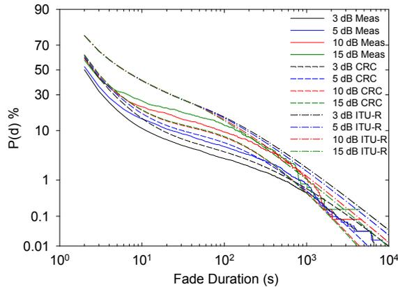
Fig. 2 Comparison of measured  $P(d)$  with results from CRC and ITU-R models for 3, 5, 10 and 15 dB fade thresholds.
