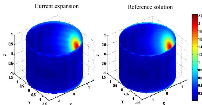
Fig.4: Comparison between a reference MoM solution and current expansion through GSF.
