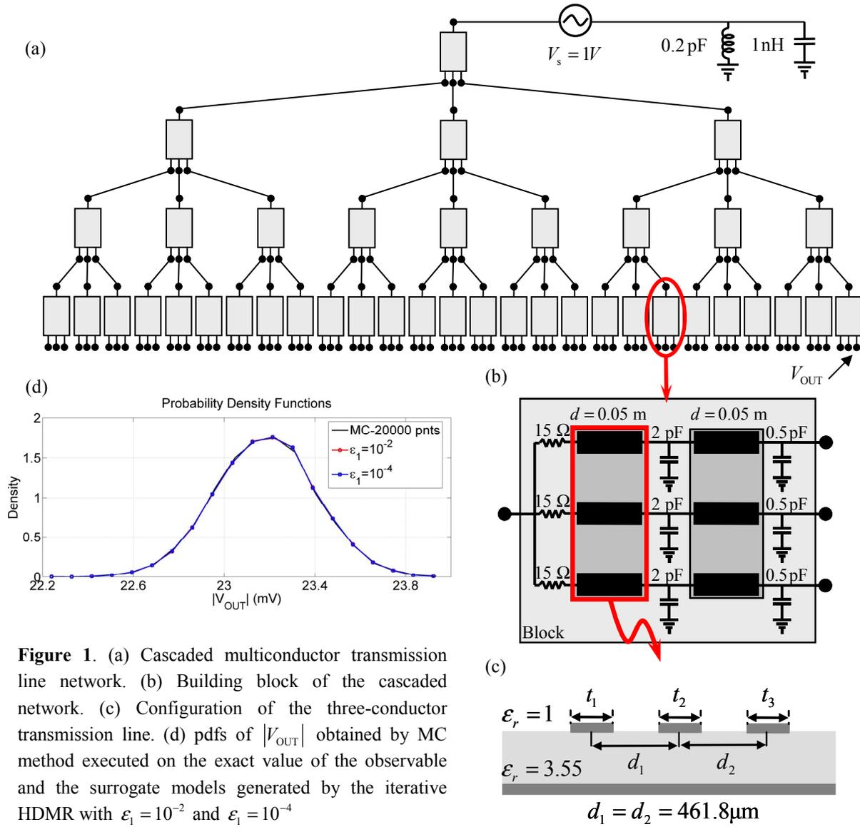
**Figure 1.** (a) Cascaded multiconductor transmission line network. (b) Building block of the cascaded network. (c) Configuration of the three-conductor transmission line. (d) pdfs of  $|V_{OUT}|$  obtained by MC method executed on the exact value of the observable and the surrogate models generated by the iterative HDNR with  $\epsilon_1 = 10^{-2}$  and  $\epsilon_1 = 10^{-4}$
