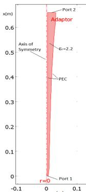
Figure 7 2-D geometry simulation setup. The exponential profile was imported in Comsol®.
