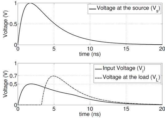
Figure 10 Simulation results. Voltage at the source, input and load. Note that the risetime of the signal at the load is preserved.
