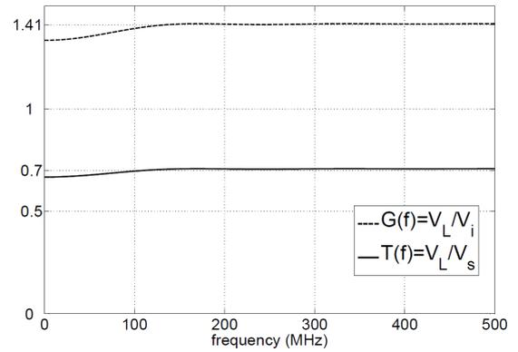
Figure 4 Magnitude of the voltage transfer functions in the frequency domain.
