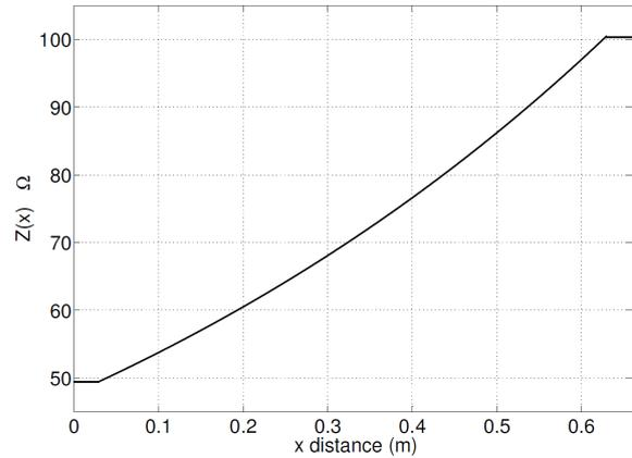
Figure 6 Impedance of the tapered transmission line along the longitudinal distance.
