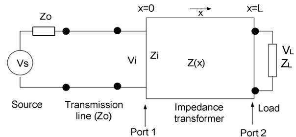
Figure 2 Circuit diagram of the Impedance adaptor.
