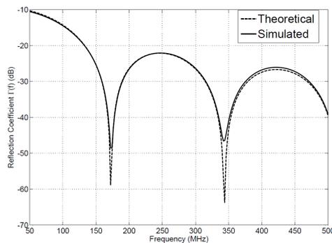
Figure 8 Simulated and analytical  $\Gamma(f)$ .
