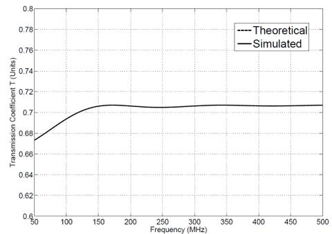
Figure 9 Transfer function  $T(f)$  obtained by numerical simulations and using Equation (8). Both graphics coincide.
