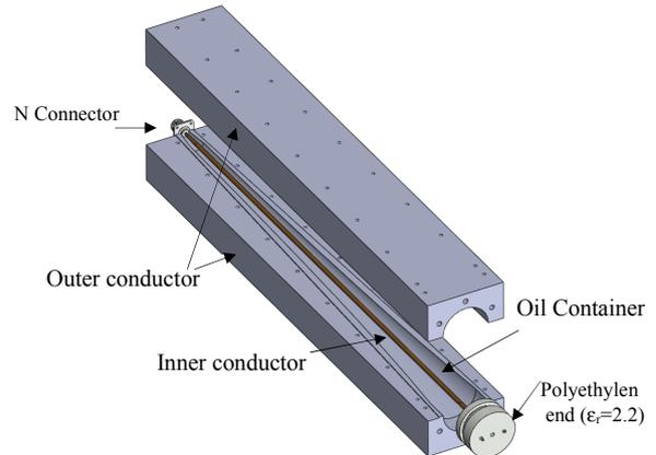
Figure 11 3-D exploded view of the exponential taper
