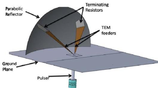
Figure 1 Half Impulse Radiating Antenna.
