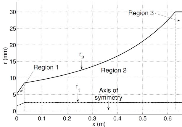
Figure 5 Profile of the taper as a function of the longitudinal distance ( $x$  and  $r$  axes are not in the same scale).
