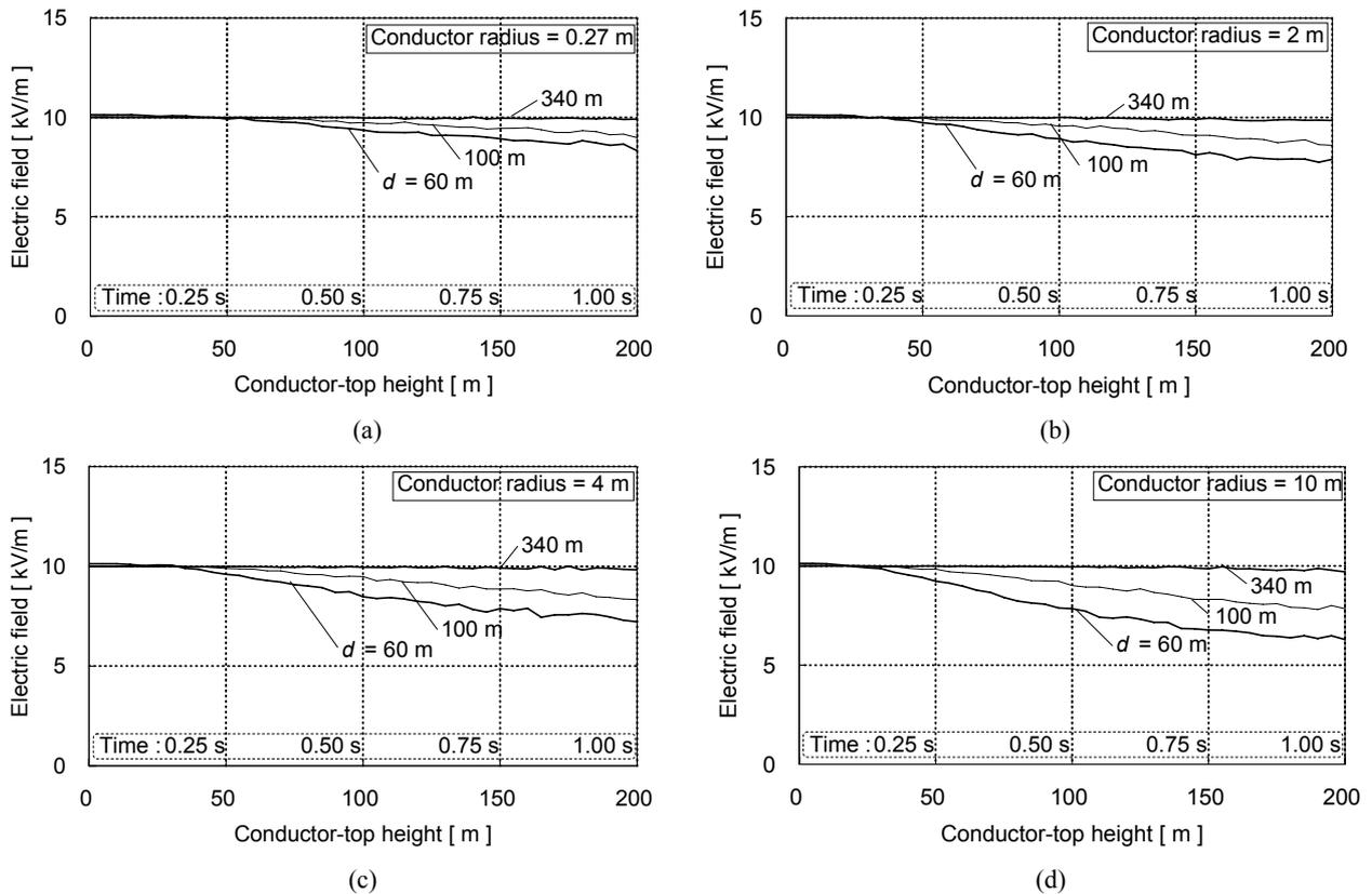
Figure 2. FDTD-calculated variations of upward-directed electric field  $E_z$  on the ground surface as a function of conductor-top height at horizontal distances of  $d=60, 100,$  and 340 m from an upward-extending conductor, for different conductor radii: (a) 0.27 m, (b) 2 m, (c) 4 m, and (d) 10 m. The conductor extends upward up to an altitude of 200 m, at a speed of  $v = 200$  m/s in a quasi-static upward-directed electric field of about 10 kV/m on the ground surface and 30 kV/m aloft.
