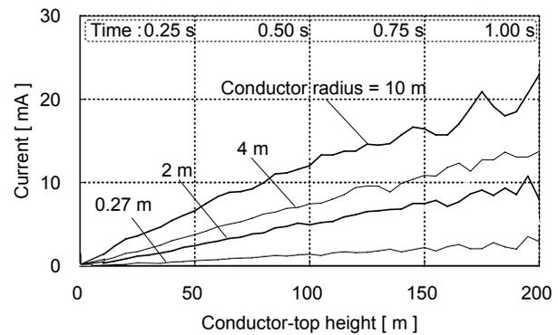
Figure 4. Currents (time derivatives of FDTD-calculated total charges shown in Figure 3) flowing in an upward-extending conductor for different conductor radii, 0.27, 2, 4, and 10 m.
