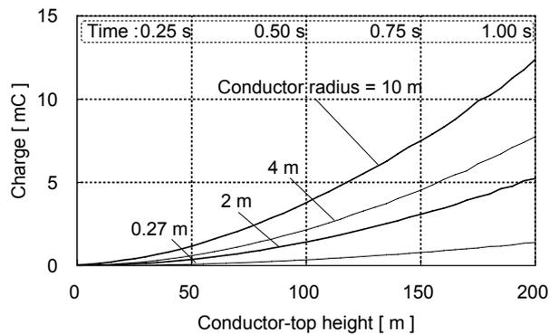
Figure 3. FDTD-calculated time-variations of total charge on the surface of an upward-extending conductor (representing both the triggering wire and its corona sheath) for different conductor radii, 0.27, 2, 4, and 10 m.
