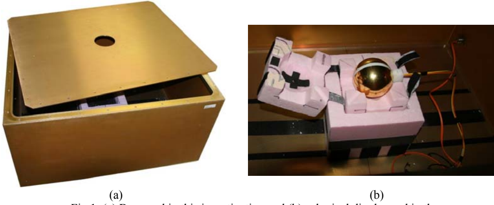
Fig 1: (a) Box used in this investigation and (b) spherical dipole used in the measurements.
