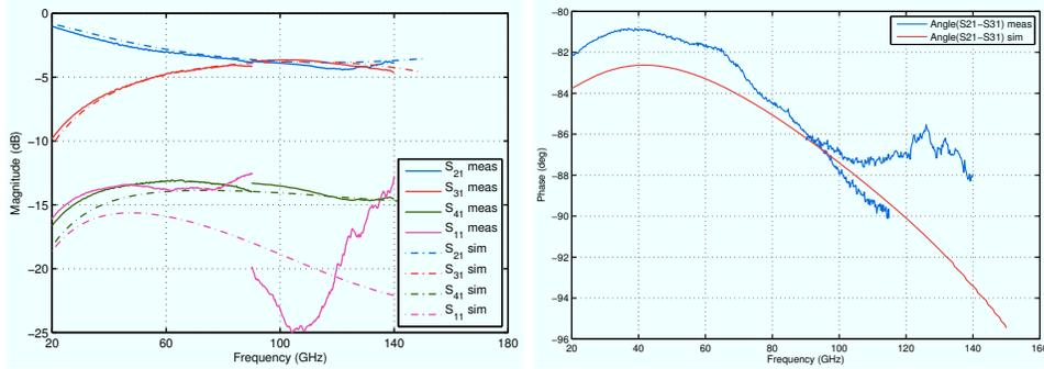
Figure 2: Comparison of S-Parameter measurement and simulation of the directional coupler.
