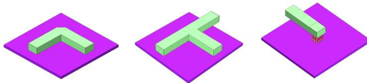
Figure 5: 3D view of modeled passive elements for subdivision of complex structures into basic elements.
