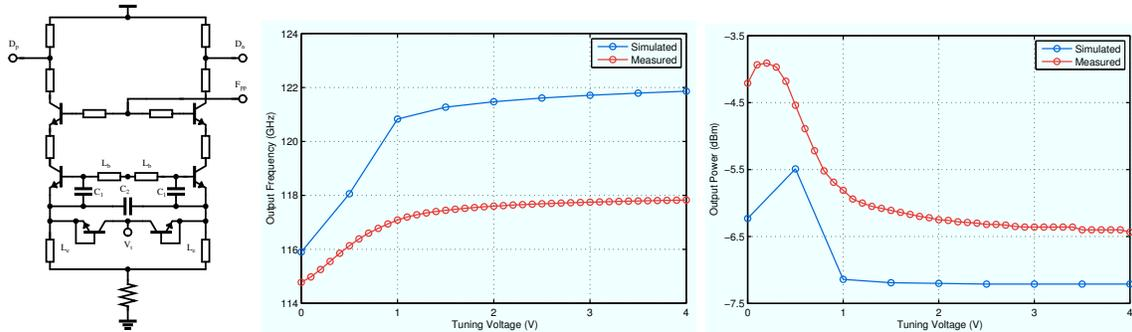
Figure 3: Schematic (left) and comparison of simulation and measurement of output frequency (middle) and output power (right) of the fabricated 116-GHz push-push VCO.
