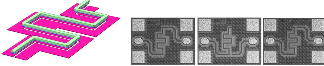
Figure 1: Layer stack (left) and simplified layout (right) of the broadside coupled directional coupler.
