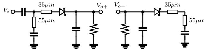
Figure 4: Schematic of the Schottky power detector for 240 GHz operation with simple L-match.
