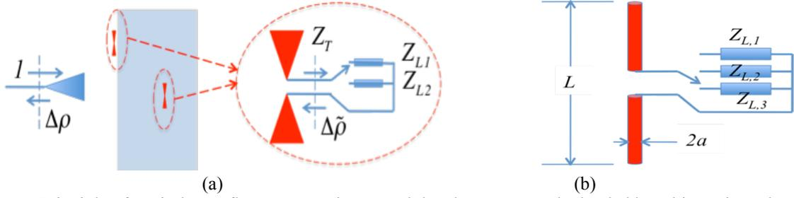
Figure 1 : Principle of a wireless reflectometer using a modulated scatterer probe loaded by a binary impedance (a), and a dipole probe loaded by a set of three impedances (b).
