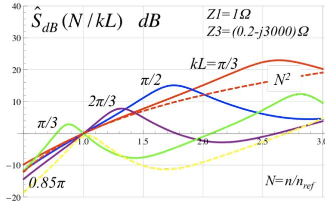
Figure 2: Normalized index sensitivity  $\hat{S}(N/kL)$  for center-loaded dipoles,  $L/a=20$
