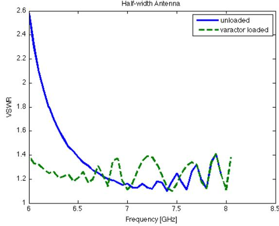
**Figure 2. Comparison of predicted VSWR between the unloaded and varactor loaded cases.**
