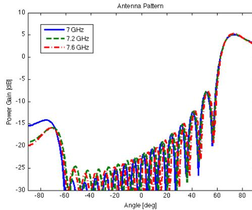
**Figure 4. Radiation patterns of a varactor loaded HWLW antenna at three different frequencies.**
