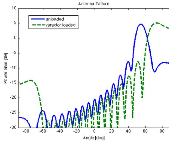
**Figure 3. Comparison of radiation patterns at 7 GHz.**
