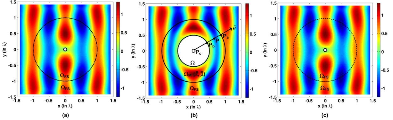
**Fig. 1.** Real part of total electric field for scattering from an electrically-small circular object: (a) Original problem, (b) Equivalent problem in original coordinates, (c) Equivalent problem after transforming the field values (in transformed coordinates) by using (2).
