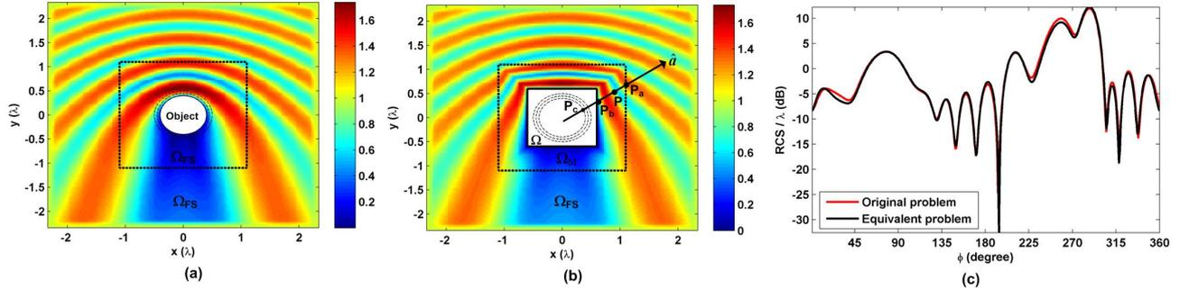
**Fig. 2.** Finite element simulation of scattering from a circular object coated by two dielectric layers: (a) Magnitude of total electric field in original problem, (b) Magnitude of total electric field in equivalent problem, (c) Radar cross section profiles.
