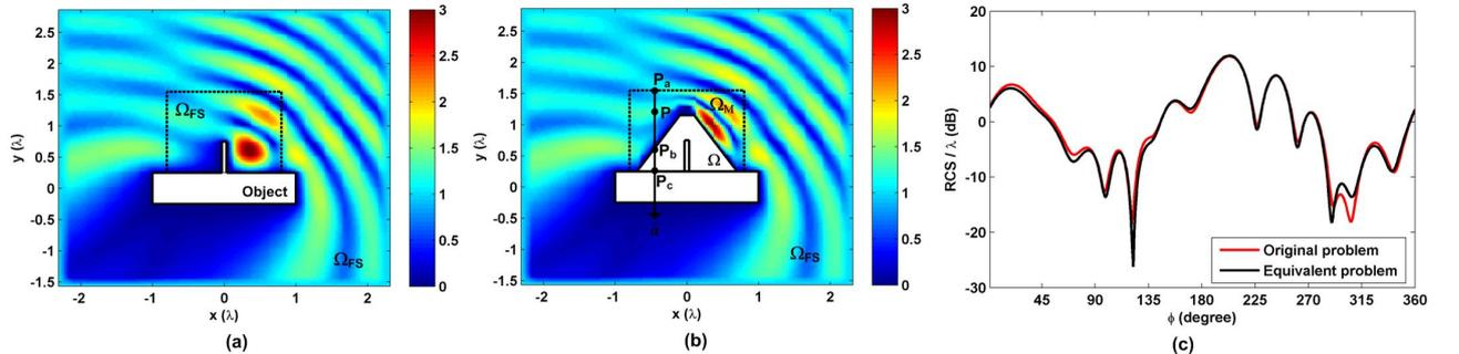
**Fig. 3.** Finite element simulation of scattering from an object with thin feature: (a) Magnitude of total electric field in original problem, (b) Magnitude of total electric field in equivalent problem, (c) Radar cross section profiles.
