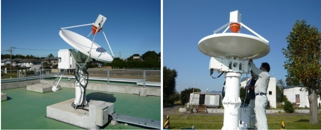
Figure 4: The MARBLE compact VLBI system with 1.6 m dish at Kashima (left) and Tsukuba (right).
