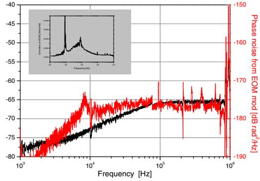
Fig. 2 Inset, EOM correction signal for phase lock comb on ultrastable laser. Black line, transfer function from EOM control to an amplitude monitoring photodiode. Redline, calculated excess phase noise induced by the unavoidable amplitude modulation cross-talk, when the EOM is serving the repetition rate.
