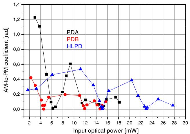
Fig. 4 AM-to-PM conversion coefficients for two DSC40s (PDA black line and PDB red line), and HLPD (blue line) from Discovery Semiconductors.
