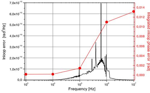
Fig. 1 Inloop error (black line) and integrated error (red line) when EOM is employed for phase lock loop.
