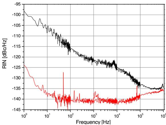
Fig. 3 Femtosecond laser comb relative intensity noise (RIN) obtained with the commercial diode laser power supply (black line), and with a home-made low noise power supply exhibiting about 3nA/rHz white noise floor (red line).
