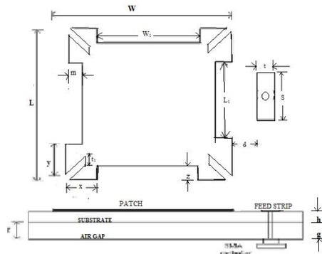
Fig.1 Geometry of novel patch antenna with small capacitive feed Strip.
