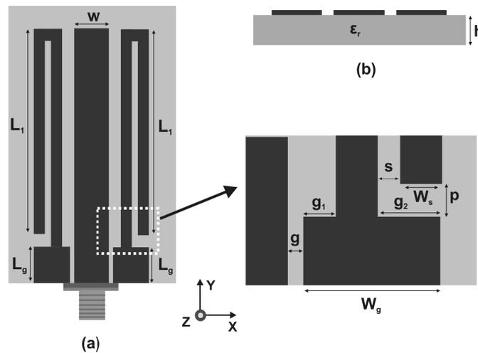
Figure. 1. Antenna geometry ( $L_1=18$ ,  $L_g=3$ ,  $w=3$ ,  $g_1=0.65$ ,  $g_2=1.5$ ,  $w_s=1$ ,  $p=1$ ,  $g=0.35$ ,  $s=1$ ,  $w_g=3.15$ ,  $h=1.6$ ,  $\epsilon_r=4.4$ (all length are in mm)) a) Front View b) Side View
