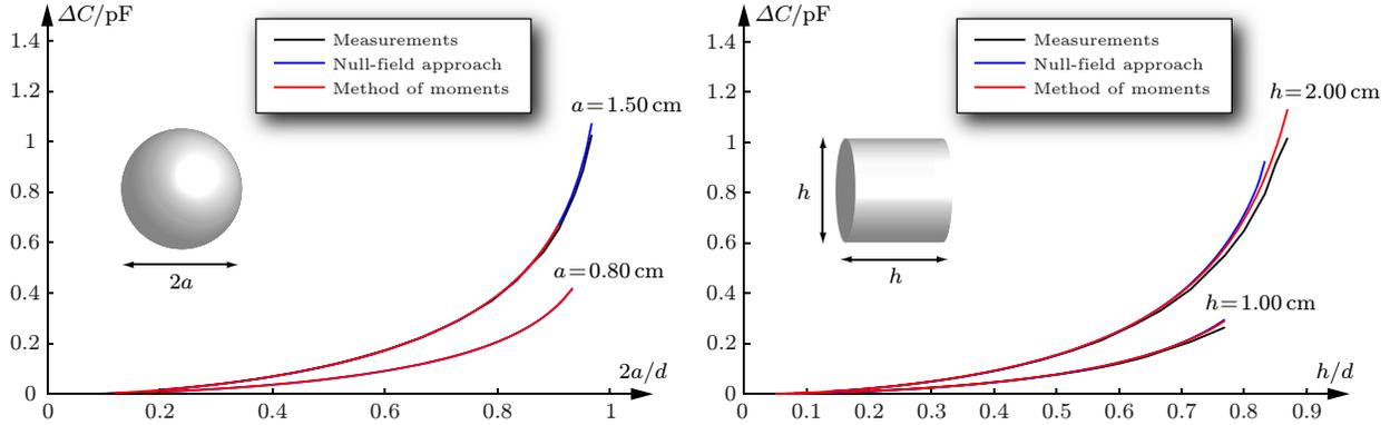
Figure 2: The change in capacitance  $\Delta C$  for a conducting sphere of radius  $a$  (left) and a circular cylinder of radius  $h/2$  and height  $h$  (right). Electrostatic measurements using the experimental setup described in Section 2 are compared to numerical simulations using the null-field approach and the method of moments.
