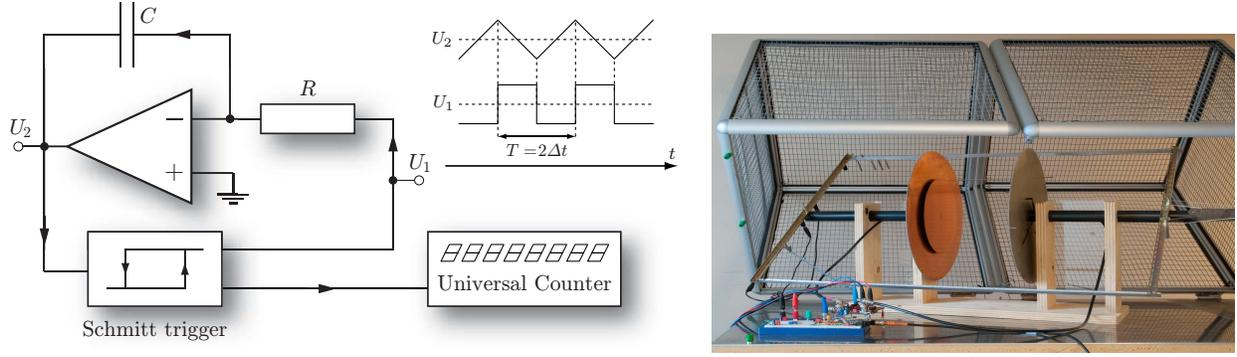
Figure 1: Block diagram of the operational amplifier circuit with voltage integrator, Schmitt trigger, and universal counter (left), and a photograph of the experimental setup (right).
