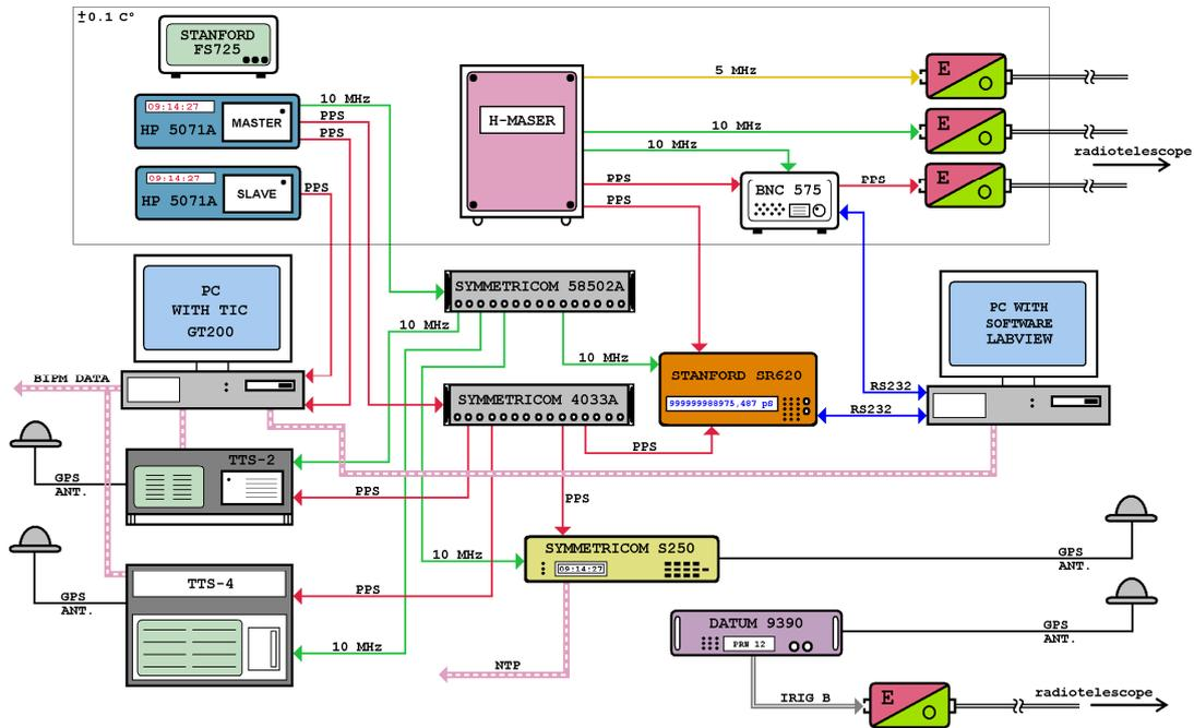
Fig. 2 – Schematic layout of the main equipments available at the T&F laboratory including both atomic resonators and ancillary devices.
