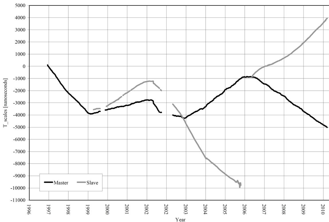
Fig. 1 – Differences between UTC and local time scale computed for the master cesium by BIPM (black curve) and for the slave cesium by an electronic counter (grey curve).
