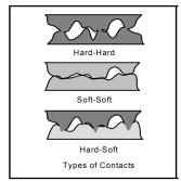
Fig. 2. Illustration of the three different types of metal contacts, showing how hard-soft contacts maximize both film penetration and contact area.
