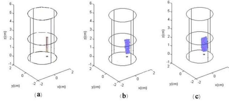
Fig.1 Comparison of the phantom reconstruction results using the data from dynamic sampling mode and step-mode, in which dynamic sampling data is acquired at the speed of  $1^\circ$  /second. (a) Original target position in the phantom. (b) 3D reconstructed result using step-mode data. (c) 3D reconstructed result using dynamic mode data at the speed of  $1^\circ$  /second.
