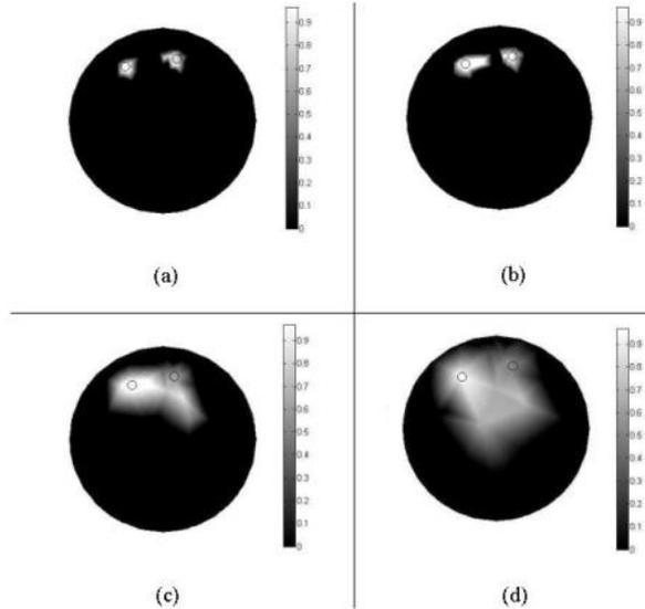
Fig.2 Comparison of the phantom reconstruction results at different rotation speeds, in which dynamic sampling data is acquired with  $6s$  exposure time of CCD. (a) Reconstructed slice with the rotation speed of  $0.5^\circ$  /s. (b) Reconstructed slice with the rotation speed of  $1^\circ$  /s. (c) Reconstructed slice with the rotation speed of  $2^\circ$  /s. (d) Reconstructed slice with the rotation speed of  $4^\circ$  /s.
