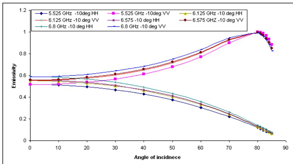
Fig 3 Variation of Emissivity of ICE with angle of incidence for different polarization and frequencies at -10 deg C and 10 deg C
