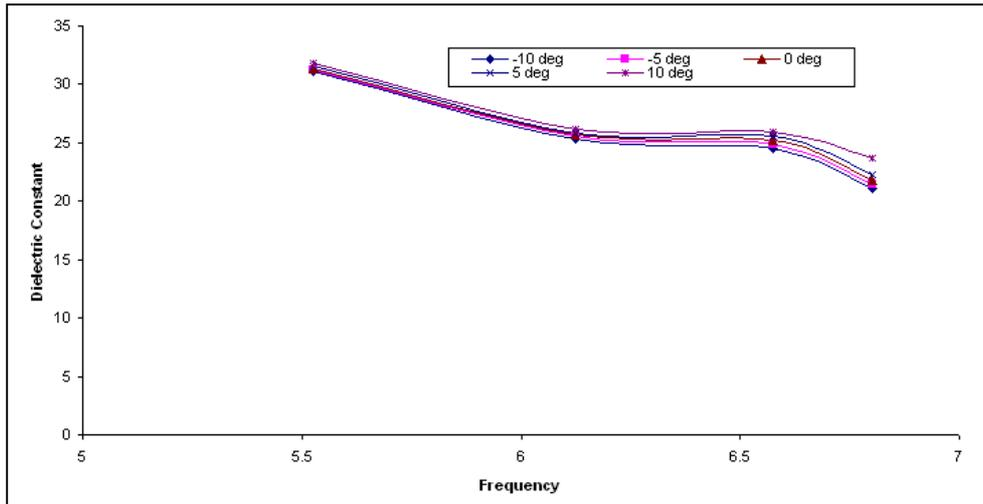
Fig 1 Variation in Dielectric constant with ICE with frequency at different Temperature
