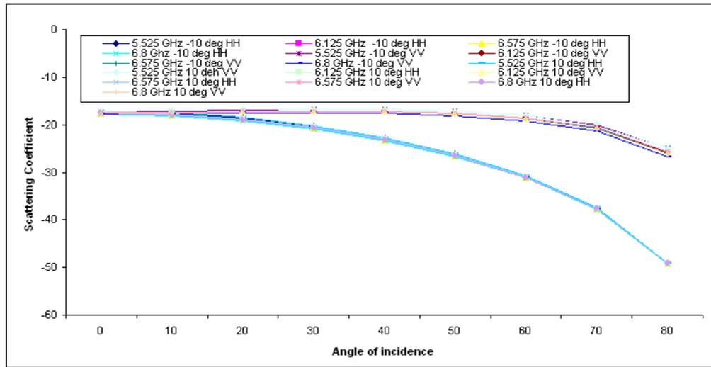
Fig 2 Variation of Scattering Coefficient of ICE with angle of incidence at different polarization and frequencies at -10 deg c and 10 deg c
