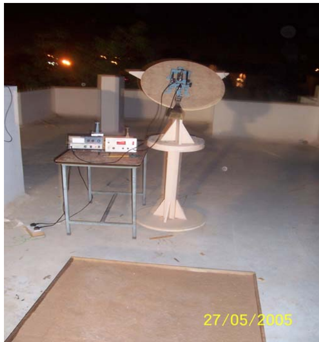
Fig. 1. Experimental set up for direct measurement of T_B using improvised Radiometer system.
