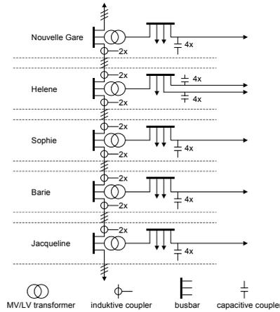
Fig. 2. Topology of the experimental network
