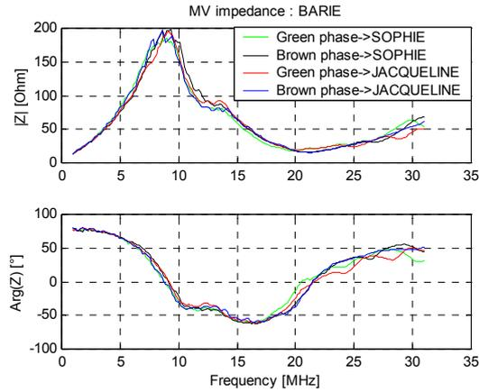
Fig. 5. Impedances of the network on the MV side
