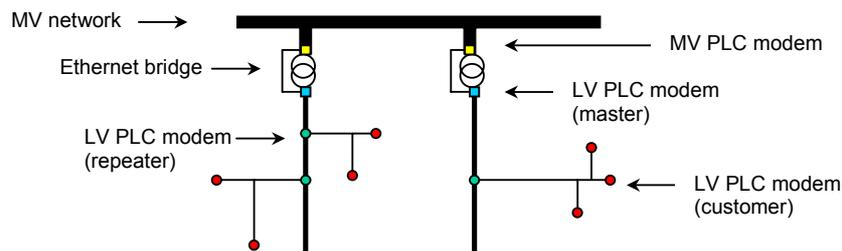
Fig. 1. PLC network using LV and MV networks
