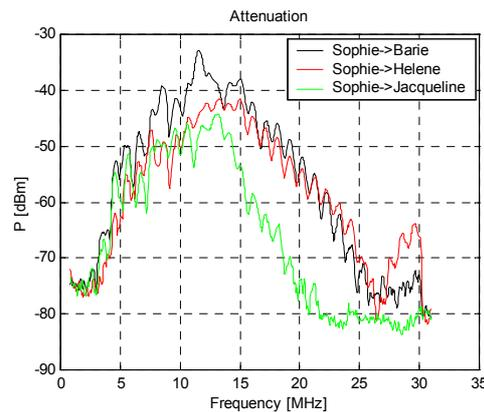
Fig. 3. Attenuation of the network on the MV side
