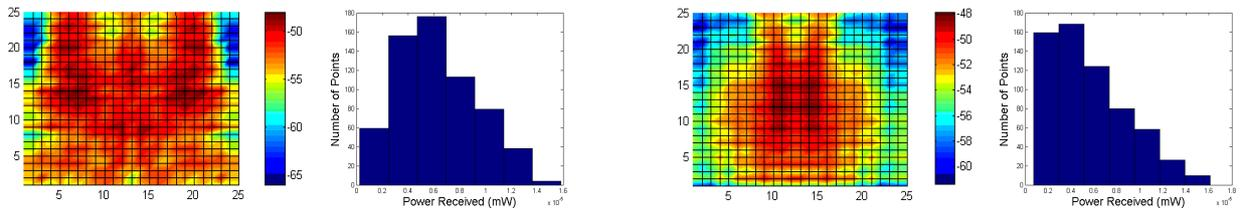
Fig. 4. The emission pattern measured and the PDF of measurement results (left); the emission pattern simulated and the PDF of simulation results (right). Planar scan; frequency: 3GHz; colormap unit for received power: dBm; unit for received power in PDF: mW; source position: 5.
