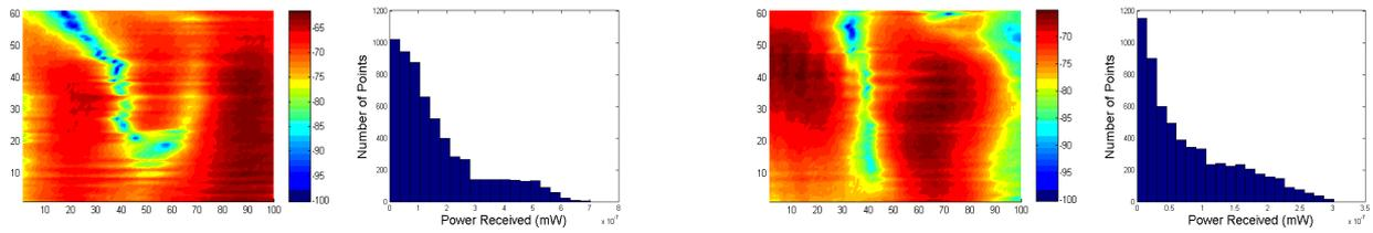
Fig. 3. The emission pattern and the PDF of received power measured as CEG02 at position 6 (left); the emission pattern and the PDF of received power measured as CEG02 at position 3 (right). Cylindrical scan; frequency: 6GHz; colormap unit for received power: dBm; unit for received power in PDF: mW.
