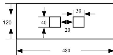
Fig. 2. Geometry of front plate with 2 slots. The slots are same in dimension. All dimensions in millimetres.
