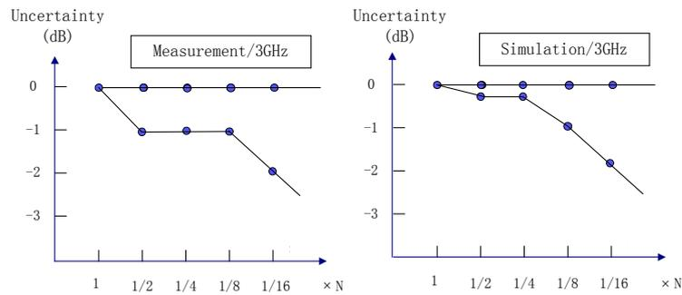
Fig. 5. Divergences of uncertainty derived from the emission patterns presented in Fig. 4.  $N=25*25$  test points.
