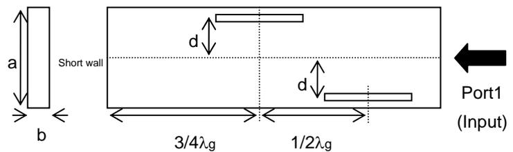
Fig.3: Parameters on the waveguide slot
