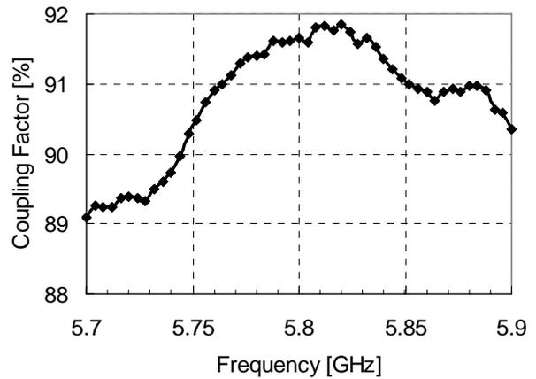
Fig.5: Measured coupling factor for Type-B
