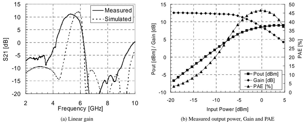
Fig.5: Characteristic of the fabricated basic amplifier
