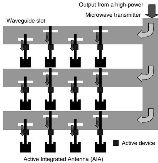
Fig.1: Concept of the Waveguide-Slot-Fed AIA
