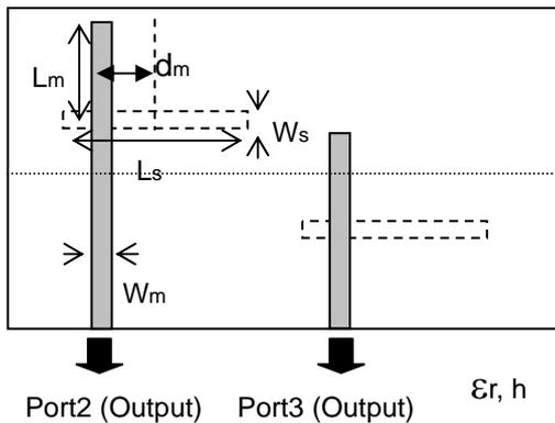
Fig.2: Parameters on the electromagnetic coupling
