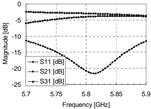
Fig.4: Measured S-parameter characteristics for type-B
