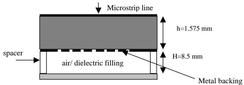
Fig .3 Cross Sectional view of the defected ground plane backed by metal plate.
