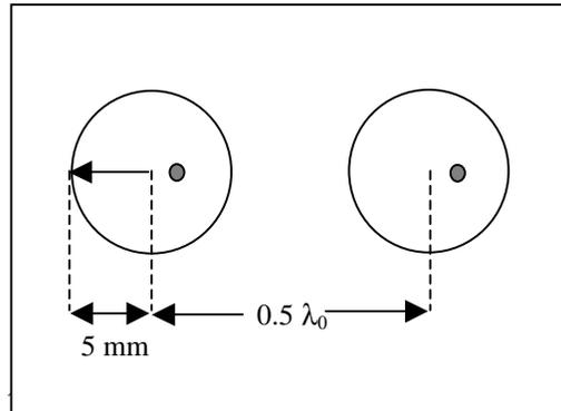
Fig .5 Two element circular patch array on a normal ground plane
