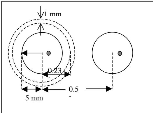
Fig .6 Two circular patch antennas separated by  $\lambda_0/2$  spacing and E-plane coupled on a defected ground plane #1.
