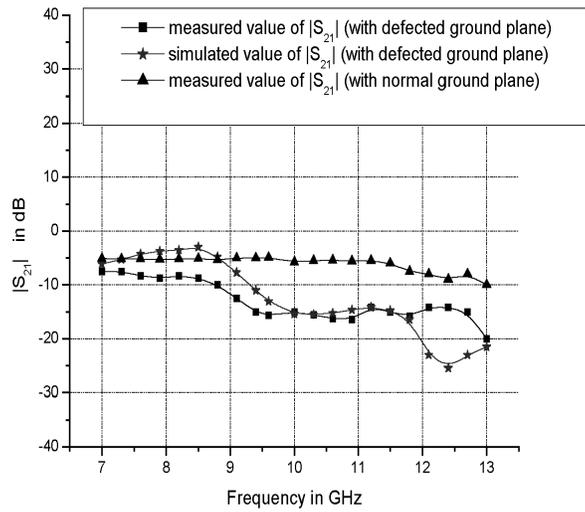
Fig.2 Measured and simulation transmission characteristics of a microstrip line with defected ground plane #1 and normal ground plane.
