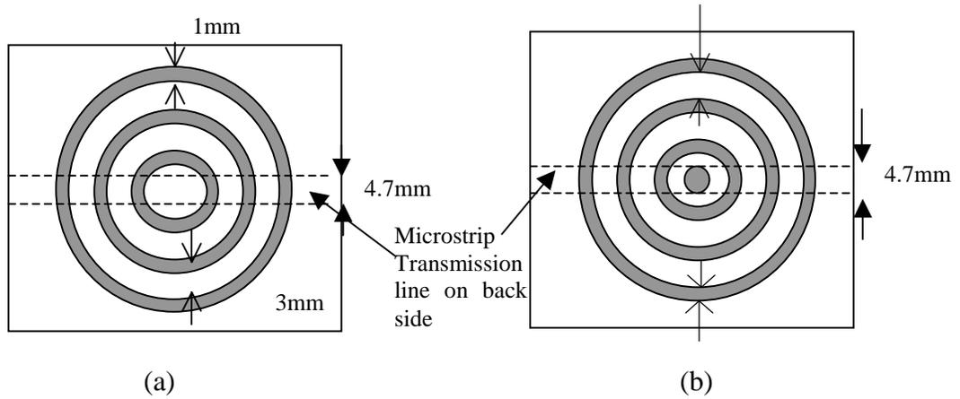
Fig .1 Front view of the defected ground plane with microstrip transmission line on the back side of a Taconic substrate of height 1.575mm and  $\epsilon_r = 2.32$ . (a) Geometry #1, (b) Geometry #2
