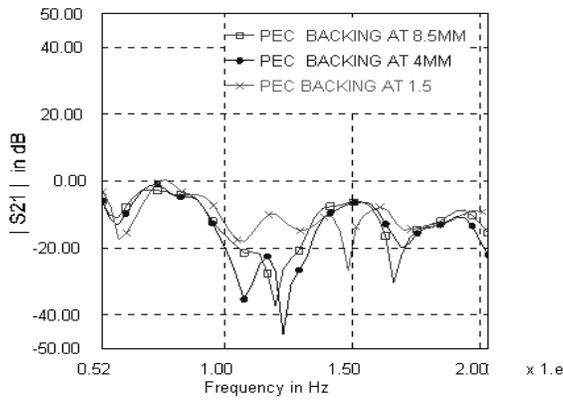
Fig. 4 Simulation data of transmission characteristics of a microstrip line with DGS #1 backed by a metal plate at three different spacing: 8.5mm, 4mm and 1.5mm and filled by air dielectric.
