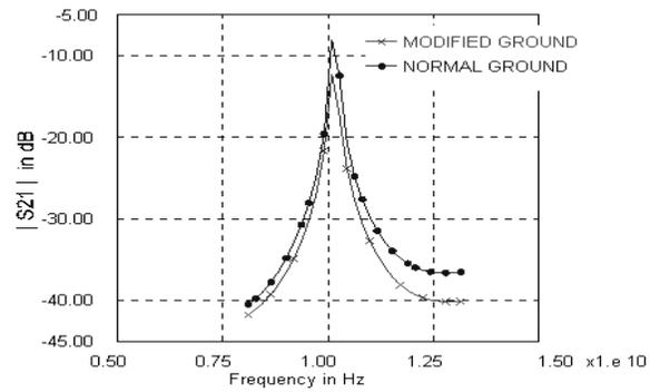
Fig .7. Simulation results of  $|S_{21}|$  for the two element arrays shown in Figs. 5 and 6,
