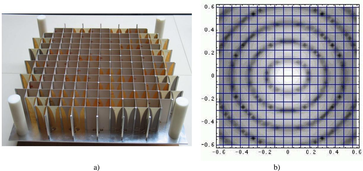
Figure 1: A prototype of a Vivaldi array similar to what will be used for PHAD is shown in a). This array operates from 1.8–6 GHz and the element spacing is 5 cm or  $\lambda/2$  at 3 GHz. In b) the array grid ( $\lambda/4$  spacing) is superimposed on the focal field distribution for the DRAO 26-m antenna (calculated using GRASP9 [13]).
