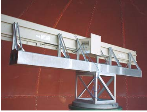
Fig. 1. The FPA antenna on its positioner inside the radome.
