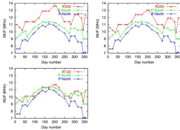
Figure 2: MUFs at 12 UT for selected quiet days in 1996 as determined from the Hankasalmi radar ground backscatter using different reflection heights (300, 250 and 120 km, corresponding to lines R300, R250 and R120 respectively) and by the PropLab program (lines P-South and P-North).
