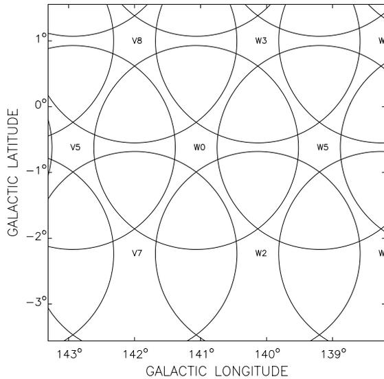
Fig 1. A schematic of the Synthesis Telescope field placements used in creating a CGPS mosaic. The radius of the fields is 93', defined by the 10% cutoff of the primary antenna beam.
