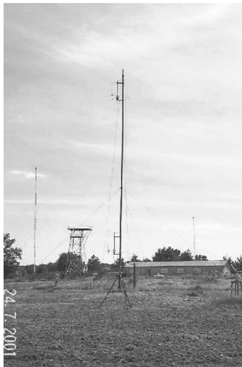
Figure 1: 2 sub arrays set up on the same mast : first sub array at 2 meters high, the second at 12 meters
