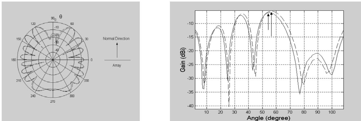
Fig. 3. Measured pattern for the active antenna array (left) and the zoom-in of the pattern around its main lobe (right). The beam steering is achieved by adjusting a RF phase shift.
