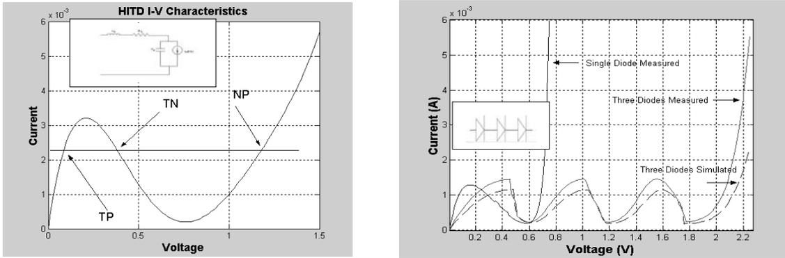
Fig. 1. (a) For a current in circuit, diodes biased in series have three possible statuses. (b) Simulated and measured I-V characteristics of the array of three tunnel diodes connected in series. Diode parameters are  $L_S=0.12$  nH,  $C_d=0.13$  pF,  $R_S=6.0$  ohm.
