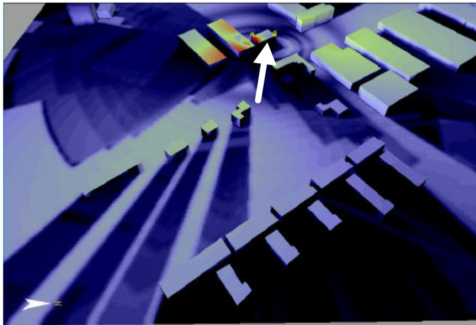
Fig.1. Field distribution around a roof mounted GSM base station (figure provided by BAKOM)
