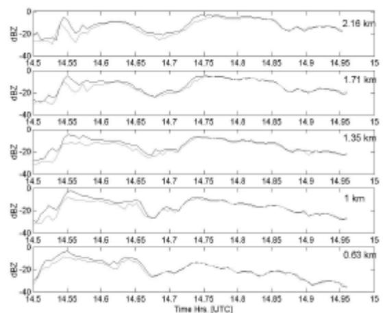
Fig. 4. Time reflectivity profiles of the 3 GHz (black curve) and 35 GHz (grey curve) at various altitudes.
