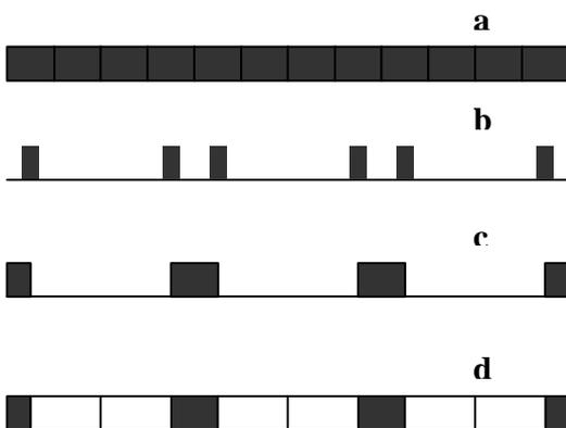
Fig. 3. Measurement schemes of the two radars spanning one minute. (a) continuous 5 s samples of the 3 GHz radar. (b) discrete 3 s samples of the 35 GHz radar. (c) Effect of integrating adjacent 35 GHz samples. (d) Using integrated 35 GHz samples to interpolate 2 samples within each measurement gap.
