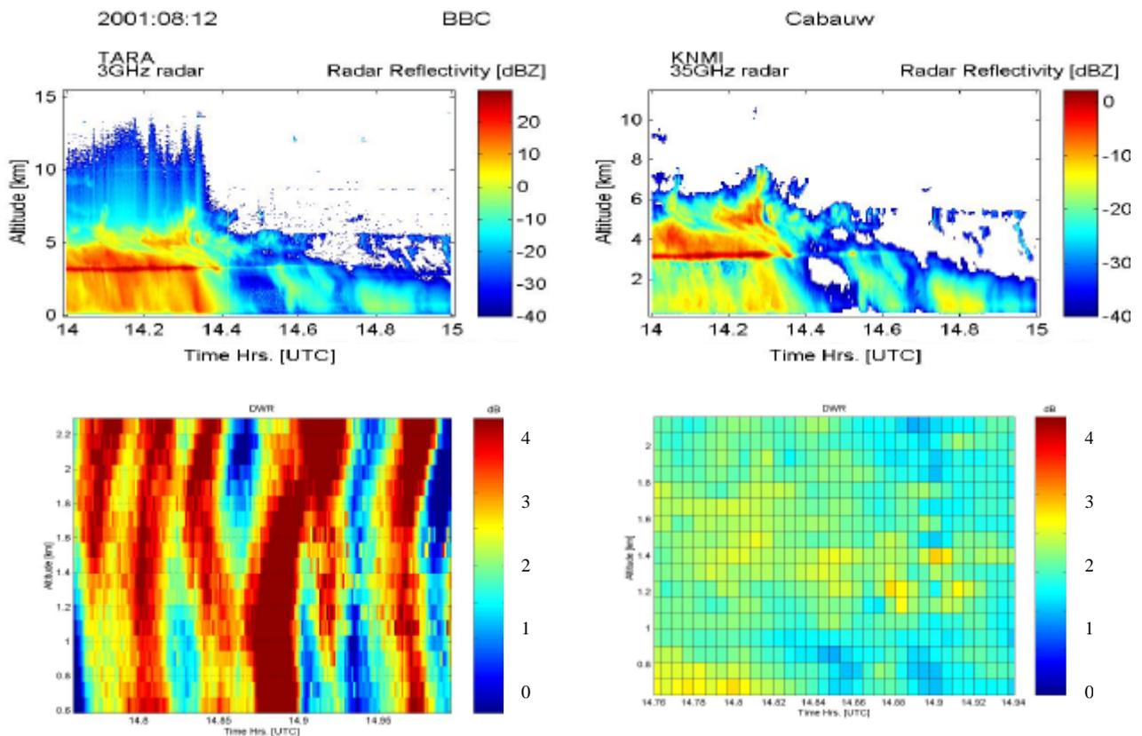
Fig. 2. Time-height sections of radar reflectivity (top two panels) of the 3 GHz radar (left), and 35 GHz radar (right). The drizzle section after 14.76 is used for the inter-comparison of the two radars. The bottom two panels show images of the DWR calculated before (left) and after (right) processing.
