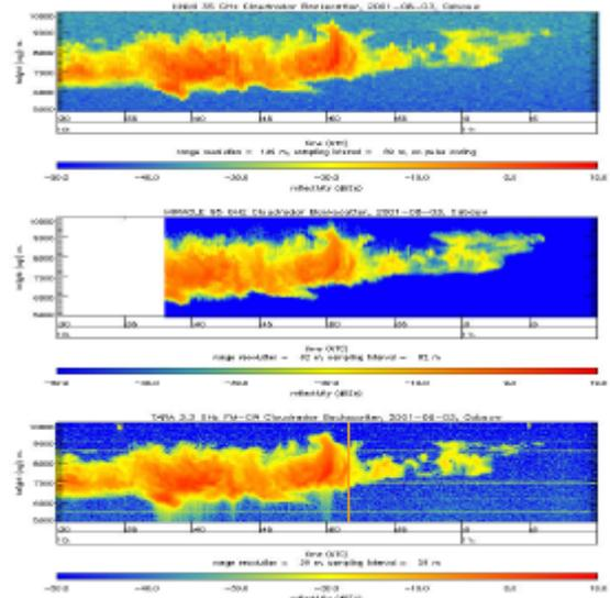
Fig. 5. Comparison of ice cloud measurements from the 3 GHz (bottom), 95 GHz (middle), and 35 GHz (top) radars.
