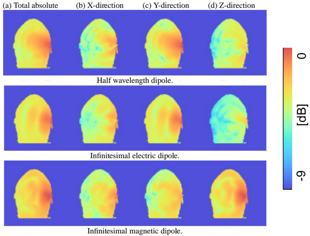
Figure 4: H-field distribution. Log scale. XY-plane. Feed in Z-direction.
