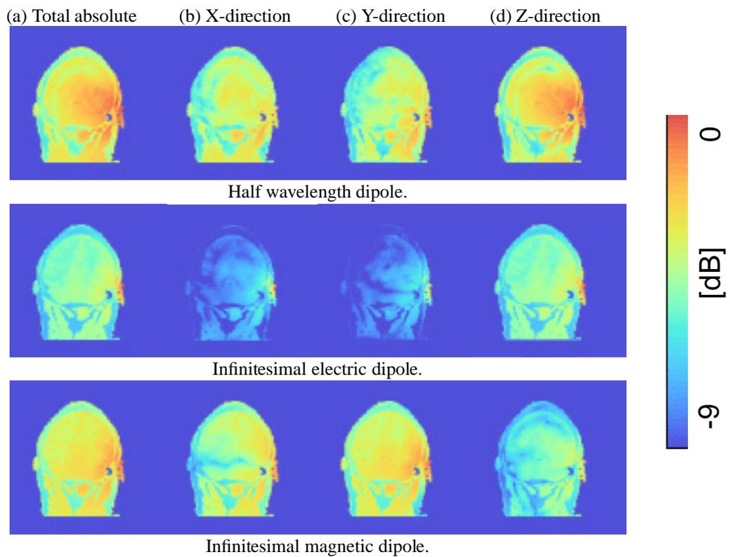
Figure 5: Current density distribution. Log scale. XY-plane. Feed in Z-direction
