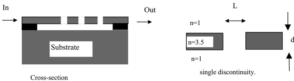
Fig. 5 - Schematic diagram of the suspended waveguide with air gaps.
