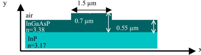
Figure 1: The transversal geometry of the simulated optical waveguide.
