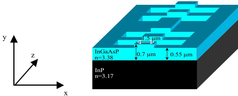
Figure 2: schematic view of studied PBG resonator.
