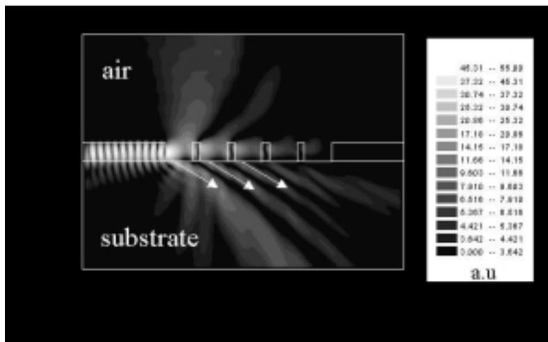
Figure 3: Field distribution for the structure described in Fig.2, calculated at  $\lambda=1.55\mu\text{m}$  using 2D-FDTD.
