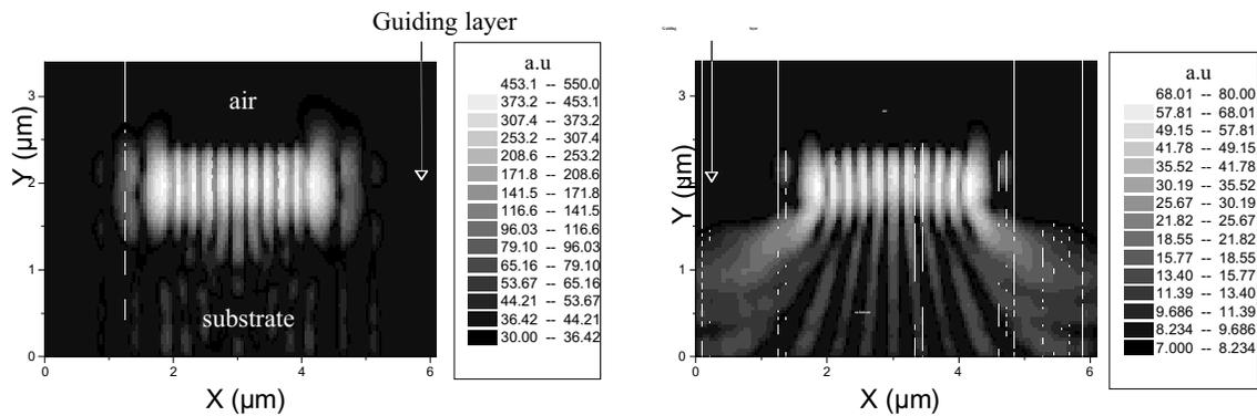
Figure 4 - Field distribution at  $\lambda=1.55\mu\text{m}$ , for the two PBG resonators investigated, using 3D-TLM.
