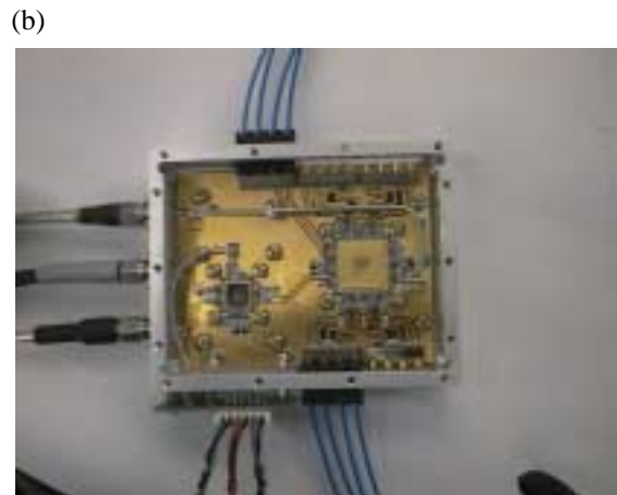
Fig. 5. (a) Block diagram of 4-Gbps 2-bit ADC system using GaAs ICs. Shaded blocks are GaAs Decision and 1:16 DMUX chips, which have been confirmed their astronomical performances. Actually the encoder part is the separate frame from the other ADC part and they are connected with SCSI cables. (b) Photograph of one set of GaAs Decision IC and 1:16 DMUX ICs. Left small IC is the Decision and right large one is the 1:16 DMUX IC. In the left side of the frame, sampling clock and analog signal are put into the printed board. Upper and lower blue cables are de-multiplexed digital signal and lower colored twisted cables are the power and ground lines.
