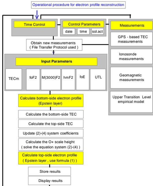
**Fig.2** Operational procedure for real-time reconstruction of the electron density distribution.
