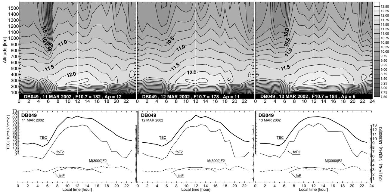
**Fig.3** Real-time reconstruction of the electron density profile, 11-13 March 2002, Dourbes (4.6°E, 50.1°N).
