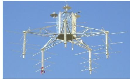
**Figure 2** : The balloon nacelle of ORAGES with the 5-antenna network.
