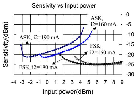
Figure 5. Sensitivity as a function of input power for both ASK and FSK receivers. Injection current to SOA 1 and CW probe power is 300 mA and 0 dBm, respectively. Injection current to SOA 2 ( $i_2$ ) is varied.
