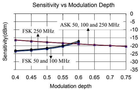
Figure 3. Sensitivity as a function of modulation depth at FSK frequency deviation of 20 GHz and for several values of laser linewidth.
