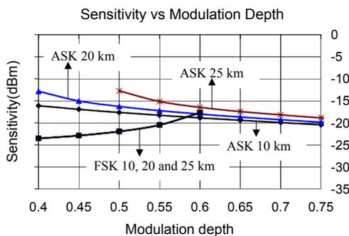
Figure 1. Sensitivity as a function of modulation depth at FSK frequency deviation of 10 GHz and linewidth of 50 MHz for several length of SMF.
