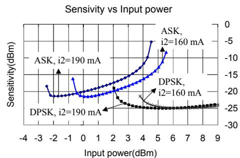
Figure 6. Sensitivity as a function of input power for both ASK and DPSK receivers. Injection current to SOA 1 and CW probe power is 300 mA and 0 dBm, respectively. Injection current to SOA 2 ( $i_2$ ) is varied.
