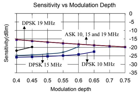
Figure 4. Sensitivity as a function of modulation depth for several values of laser linewidth.
