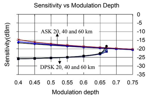
Figure 2. Sensitivity as a function of modulation depth at linewidth of 10 MHz for several length of SMF.
