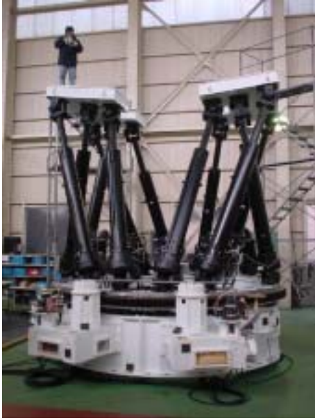
Figure 2: (left) Dual-beam platform system. Receivers are installed on the Steward-mount platform supported by six arms.
