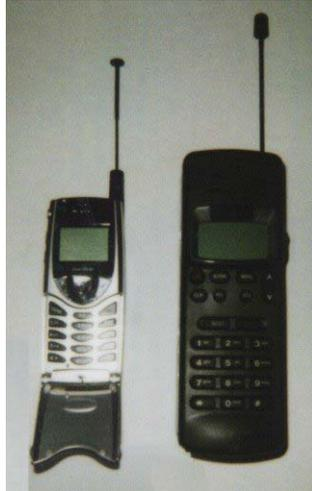
Fig. 1. Two commercial telephones A (left side) and B (right side) selected for SAR testing at 835 MHz.
