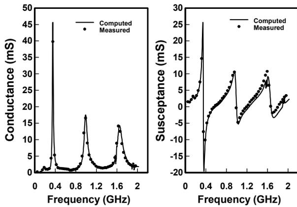
Fig. 7: Input admittance for  $\rho_c = 6.5$  cm,  $L = 22.38$  cm,  $h_c = 28.02$  cm,  $\rho_o = 4.915$  cm
