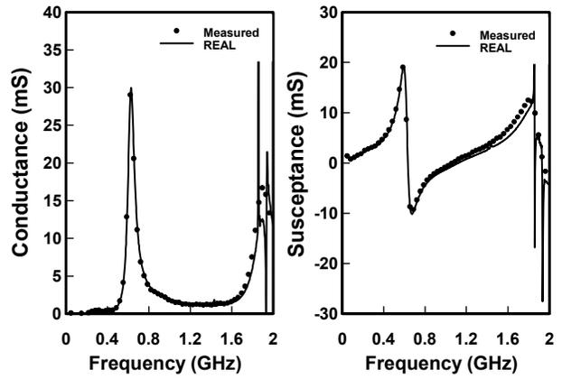
Fig. 6: Input admittance for  $\rho_c = 6.5$  cm,  $L = 11.47$  cm,  $h_c = 17.5$  cm,  $\rho_o = 4.915$  cm
