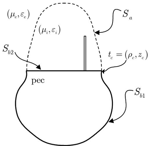
Fig. 1: Antenna attached to a conducting body
