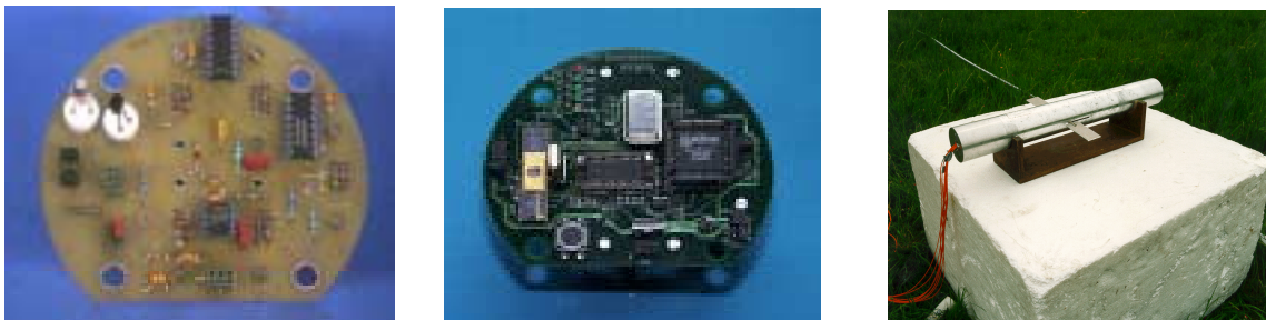
Figure 1: Printed circuit boards used for HPM-testing integrated in GENEC missile dummy
