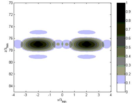
Fig. 3. Amplitude reconstruction of two pulses with  $a=25\lambda_{\min}$  and located at  $(-2\lambda_{\min}, 77\lambda_{\min})$  and  $(2\lambda_{\min}, 77\lambda_{\min})$
