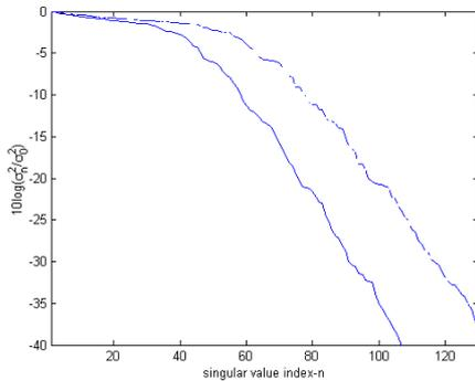
Fig. 2. Normalized behaviour of the singular values; solid line  $a=25\lambda_{\min}$ ; dashed line  $a=35\lambda_{\min}$
