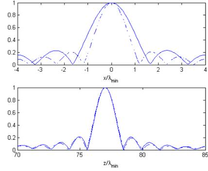
Fig. 5. Amplitude reconstruction of a pulse located at  $(0,77\lambda_{\min})$ . Cut along  $x$  (top); Cut along  $z$  (bottom);  $a=25\lambda_{\min}$  (solid line);  $a=35\lambda_{\min}$  (dashed line)
