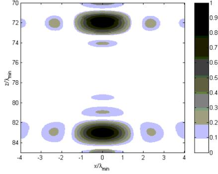
Fig. 4. Amplitude reconstruction of two pulses with  $a=25\lambda_{\min}$  and located at  $(0,72\lambda_{\min})$  and  $(0,83\lambda_{\min})$
