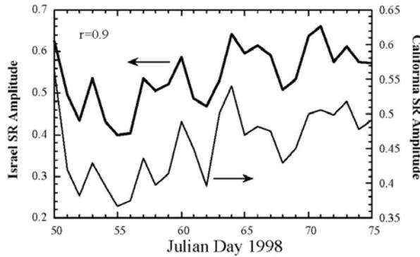
Figure 1: The simultaneous daily measurements of the 8 Hz horizontal magnetic field amplitude in Israel and California.
