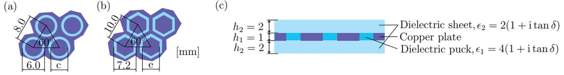
Fig. 4. Two examples of FSS patterns; (a) annular FSS, (b) hexagonal FSS. In (c) the vertical cross-section of an FSS is depicted. Annular 1 has  $c = 5.0$  mm, while annular 2 has  $c = 4.0$  mm. The hexagonal FSS has  $e = 5.2$  mm.
