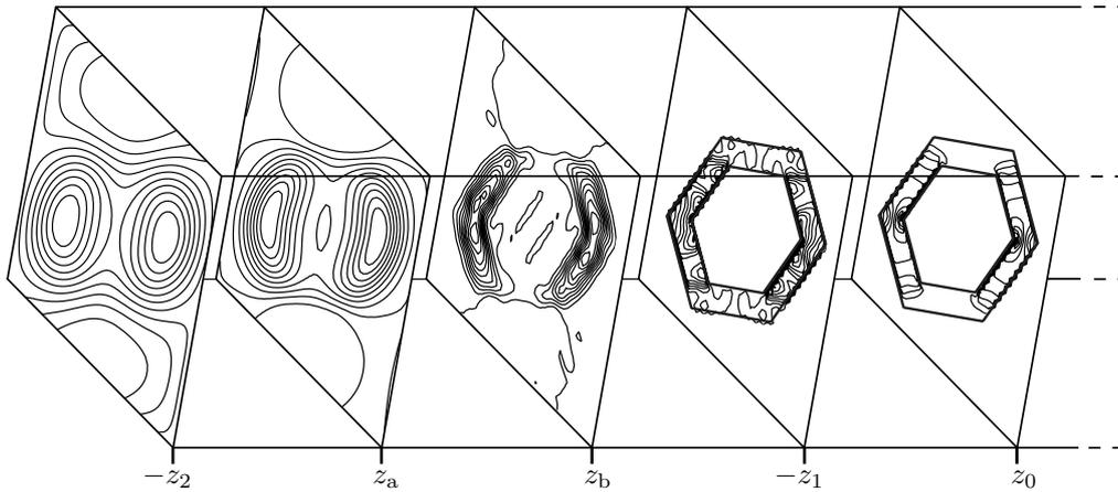
Fig. 3. Power flow density for a symmetric hexagonal FSS, cf., Fig. 2.
