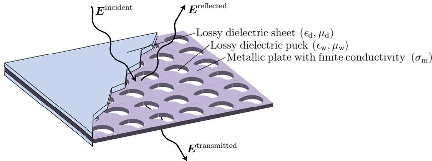
Fig. 1. A Thick Frequency Selective Structure (FSS).
