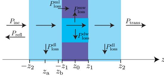
Fig. 2. Power flow through a FSS.
