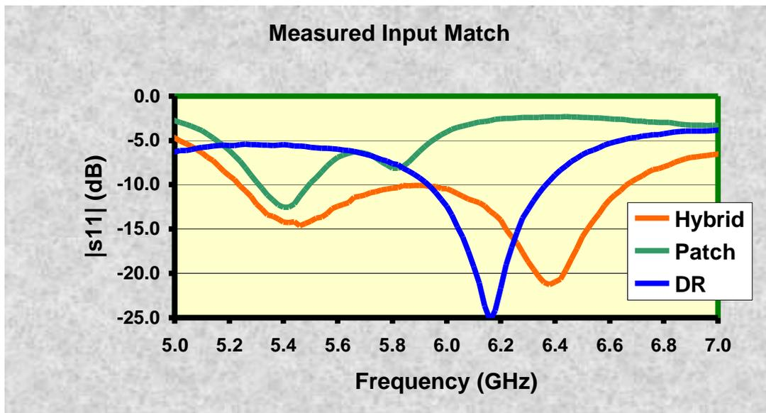
Fig. 2. The measured input return loss of the hybrid antenna is shown in red. Other curves show the return loss of the individual dielectric-resonator antenna and the patch antenna.
