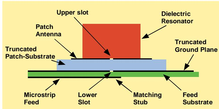
Fig. 1. The hybrid antenna configuration
