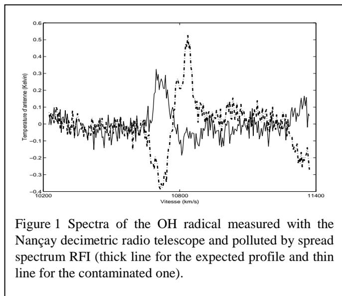
Figure 1 Spectra of the OH radical measured with the Nançay decimetric radio telescope and polluted by spread spectrum RFI (thick line for the expected profile and thin line for the contaminated one).
