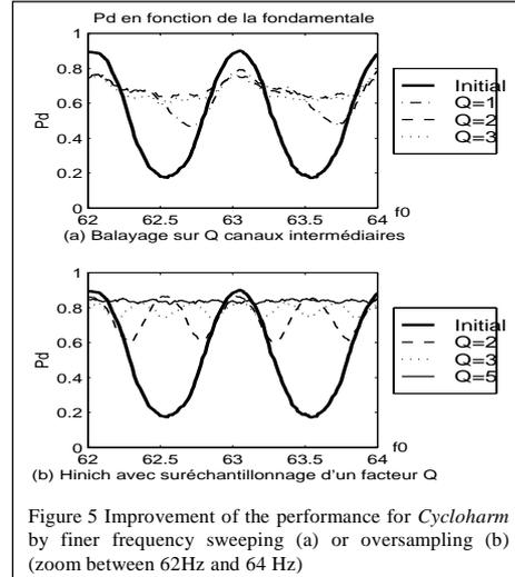
Figure 5 Improvement of the performance for *Cycloarm* by finer frequency sweeping (a) or oversampling (b) (zoom between 62Hz and 64 Hz)
