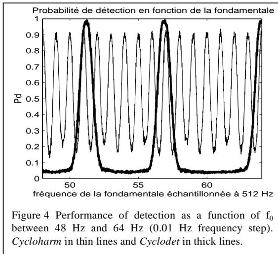
Figure 4 Performance of detection as a function of  $f_0$  between 48 Hz and 64 Hz (0.01 Hz frequency step). *Cycloarm* in thin lines and *Cyclodet* in thick lines.
