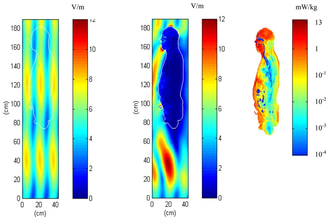
Fig 1 Field and SAR distributions, on the vertical plane containing the antenna maximum radiation direction, for the subject positioned on the balcony in front of the building where the antenna is located.
