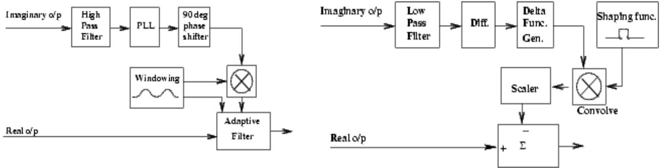
Figure 3: Block diagram of the color burst (left) and synch signal (right) suppressors.
