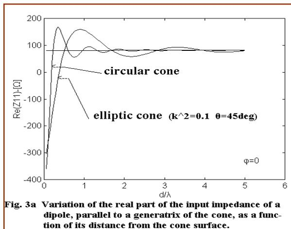
Fig. 3a Variation of the real part of the input impedance of a dipole, parallel to a generatrix of the cone, as a function of its distance from the cone surface.
