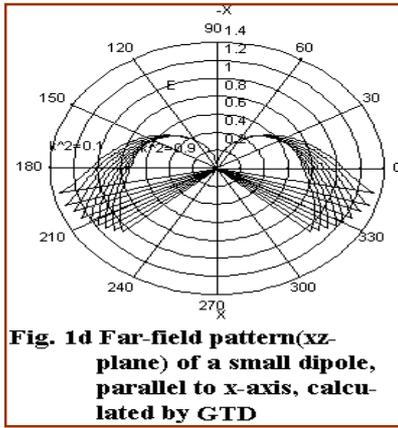
Fig. 1d Far-field pattern (xz-plane) of a small dipole, parallel to x-axis, calculated by GTD
