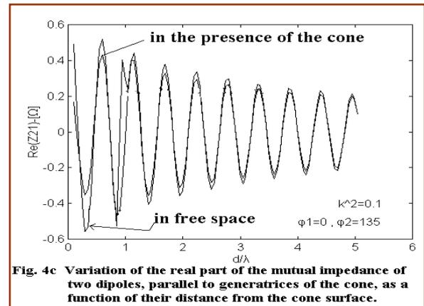
Fig. 4c Variation of the real part of the mutual impedance of two dipoles, parallel to generatrices of the cone, as a function of their distance from the cone surface.
