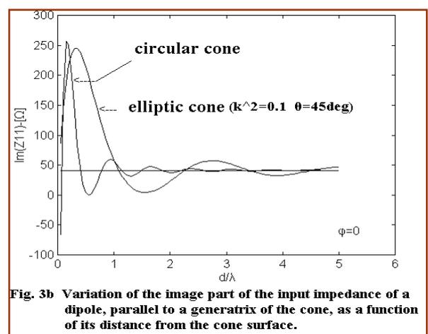
Fig. 3b Variation of the image part of the input impedance of a dipole, parallel to a generatrix of the cone, as a function of its distance from the cone surface.
