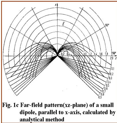
Fig. 1c Far-field pattern (xz-plane) of a small dipole, parallel to x-axis, calculated by analytical method
