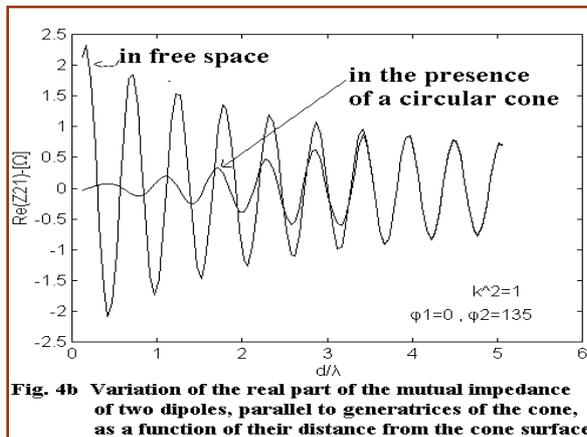
Fig. 4b Variation of the real part of the mutual impedance of two dipoles, parallel to generatrices of the cone, as a function of their distance from the cone surface
