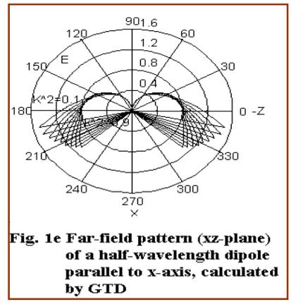
Fig. 1e Far-field pattern (xz-plane) of a half-wavelength dipole, parallel to x-axis, calculated by GTD
