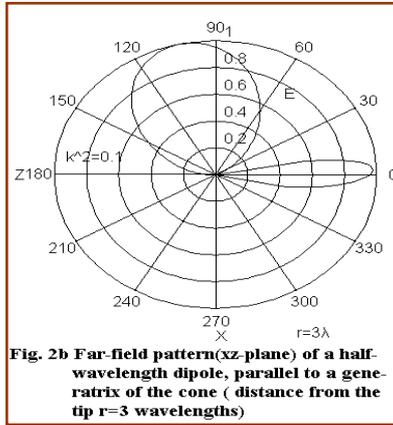
Fig. 2b Far-field pattern (xz-plane) of a half-wavelength dipole, parallel to a generatrix of the cone ( distance from the tip  $r=3$  wavelengths)
