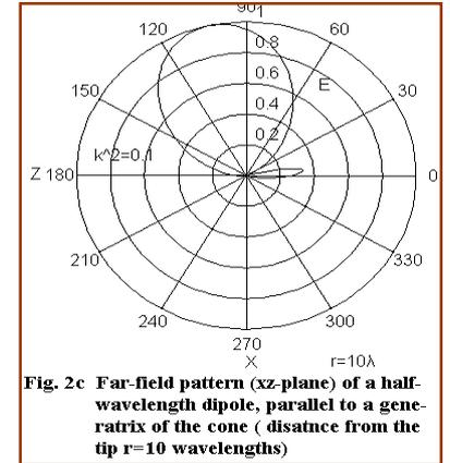
Fig. 2c Far-field pattern (xz-plane) of a half-wavelength dipole, parallel to a generatrix of the cone ( distance from the tip  $r=10$  wavelengths)
